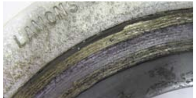
Lamons WRI-HTG spiral wound gasket after exposure to 1500°F - Maintaining the proven and superior sealing characteristics of flexible graphite creates an ideal high temperature solution - the flexible graphite is completely protected from oxidation.
