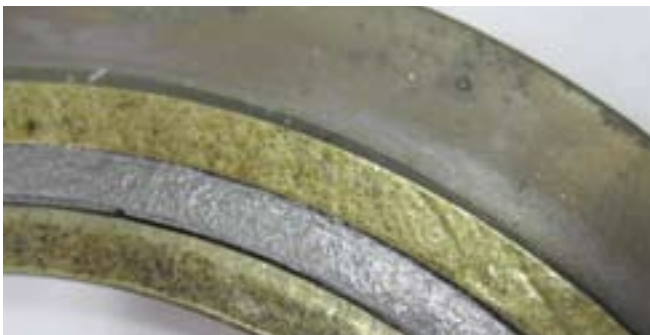
Lamons Kampro HTG after exposure to 1500°F - The flexible graphite maintains all its physical and mechanical properties after exposure.
