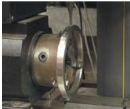
All Ring Type Joints are engraved on the nonseating surface with the ring number, heat number, material identification and the API licence number.
